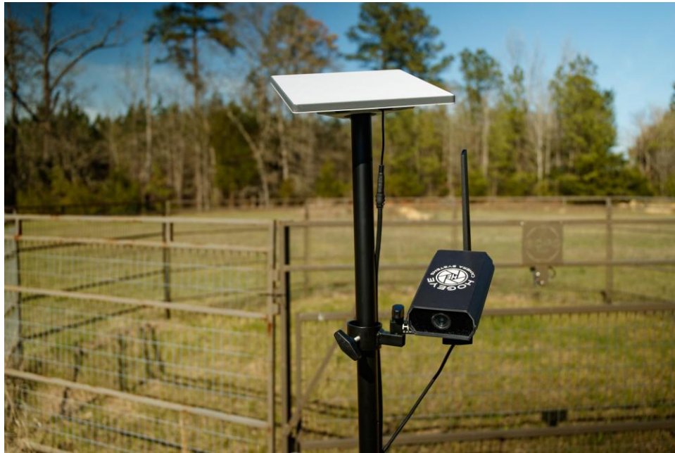
Field deployment: Starlink Mini mounted on top of the included freestanding stand with the HogEye camera mounted on the side.
